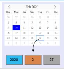
8. [History Data Added watch feature. By tapping on a record in History Data Display object, data in the selected row can be output to the designated addresses. This setting can be found in the General tab in the object settings window.
