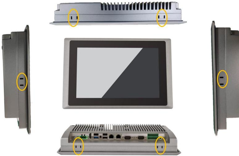
VESA75 installation, in the back of the machine, designed a standard VESA75 mounting hole position, using this way of installation requires a VESA75 bracket
