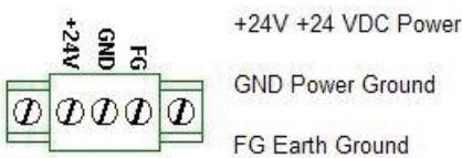
To make a connection, strip about 3/8" of insulation off the end of the wire, turn the connector screw counterclockwise until the gap is wide open, insert the wire all the way in, and turn the screw clockwise until it's tight.
