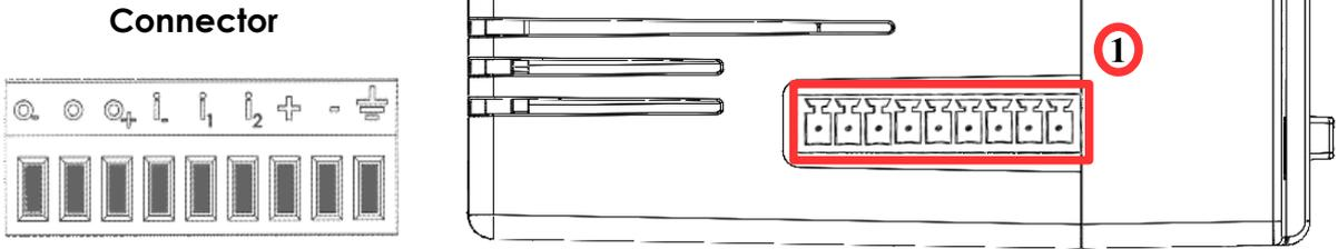
1 Main connector including power input terminal, 1DO and 2 DI
