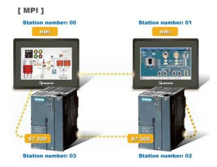
For SIEMENS S7-300 MPI driver in Multi-HMIs-Multi-PLCs communication, [Max. station no. (MPI network)] parameter must be correctly set. This setting is relevant to the station no. of the devices, as shown, two HMI (station no. 0, 1) and two PLC (station no. 2, 3) are in MPI network, Max. Station No. should be set to 3.
