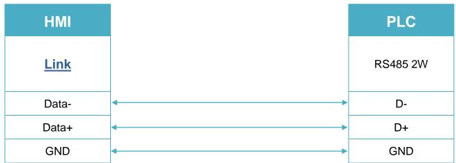
Note: Setting more than one Modbus Server in HMI Device List is of no effect.
