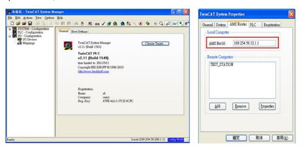
c. Use Twincat to build a Route Table to make sure the system is connected, if PLC power turns OFF and then ON, please redo this step.
