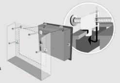
2.6 ~ 3.9 lbf.in. (For reaching waterproof effect and preventing the panel from being deformed.) Plan for adequate space around the unit and inside the enclosure, for ventilation and cables. Consider the heat from other devices inside the enclosure. The ambient temperature around the unit must be  $0 \sim$
