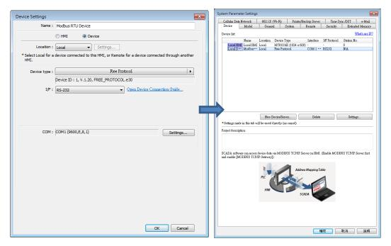
The interface of the device (I/F) uses [RS-232]. If a MODBUS TCP/IP device is connected, the interface should be [Ethernet] with correct IP and port number as follows:
