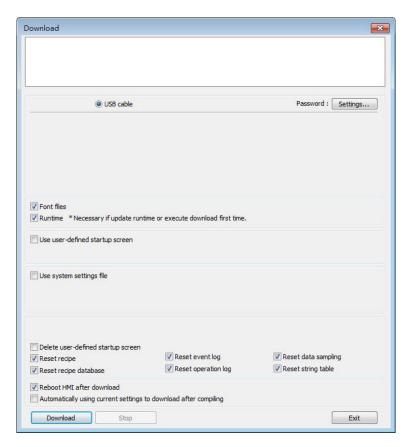
Select USB cable to download project to HMI. The way of setting is same as "3.6.1 Configure in EasyBuilder Pro". Before downloading via USB cable, please make sure the USB driver is installed. Go to [Computer Management] » [Device Manager] to check if USB driver is installed. If it is not installed, please refer to installation steps to install manually.
