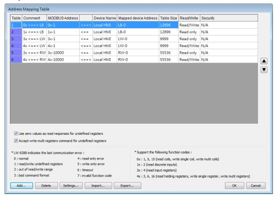
4. In the example below, to access the data in the 50 consecutive registers of FATEK FB Series PLC starting from register D-0, configure the settings as shown in the following figure.
