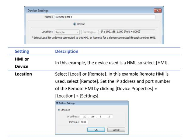
After all settings are completed, a new device named "Remote HMI 1" is added to the [Device list].
