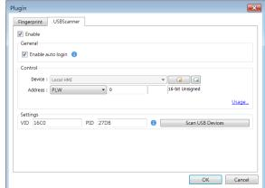
When configuring the USB scanner, to prevent interference from other USB devices during login, it's necessary to first set the VID and PID of the USB scanner. After clicking [Scan USB Devices], the system will prompt a message "Please insert your USB Device". Once the USB scanner is inserted into the PC, the system will obtain a unique VID and PID for the USB scanner. Click [Save], and the system will automatically incorporate this VID and PID into the settings.
