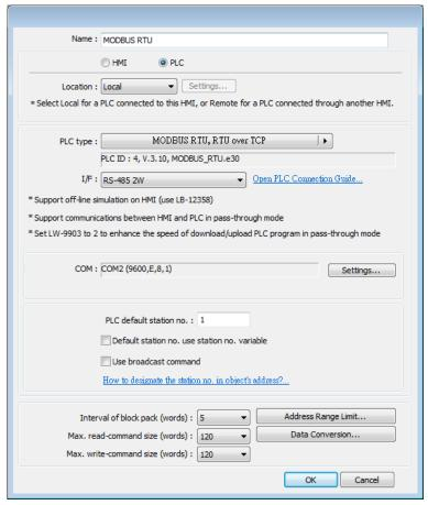
2. When finished, click [OK], then a new device "MODBUS RTU" is listed in the [Device] tab.
