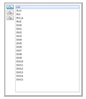
Data in the extended memory is saved as a file into [SD card] or [USB disk]. By default, the files in [EM0] to [EM15] are with the file names "em0.emi" to "em15.emi" respectively, although users are free to change the file names. To open these files and edit the data in the extended memory, RecipeEditor.exe may be used.
