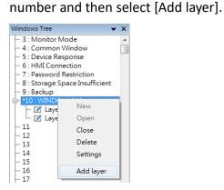
The following is an example of creating a layered window: Place a Bit Lamp object in Layer 1 and a Numeric object in layer 2.
