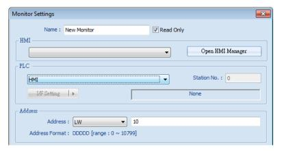
**4.** When a Word address is selected, set the address type to [Numeric] or [String]. [Numeric]: Select the data format of the monitor address.
