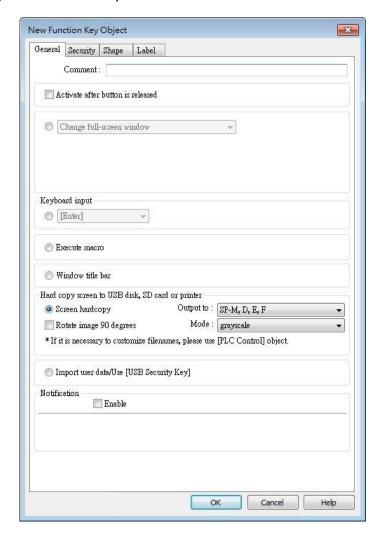
Or, use PLC Control [Screen hardcopy] to start printing with a designated bit address.
