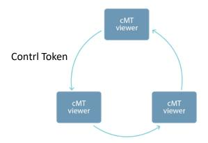
One cMT / cMT X HMI can be simultaneously controlled by multiple cMT Viewer clients. To ensure system safety by preventing an object to be controlled by multiple clients simultaneously, a control token can be set. Only one cMT Viewer client can acquire the control token at a time, and only the cMT Viewer client that acquires control token can operate the object. The rest of the clients can acquire the token one by one when the token is not occupied.
