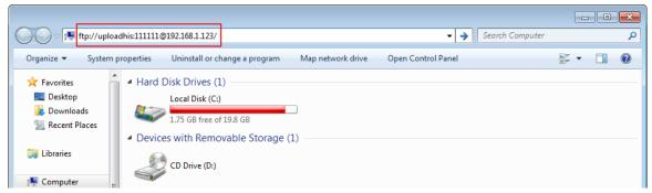
3. After entering the IP address, the ftp address: <a href="ftp://192.168.1.123">ftp://192.168.1.123</a> and its folders are shown as below:
