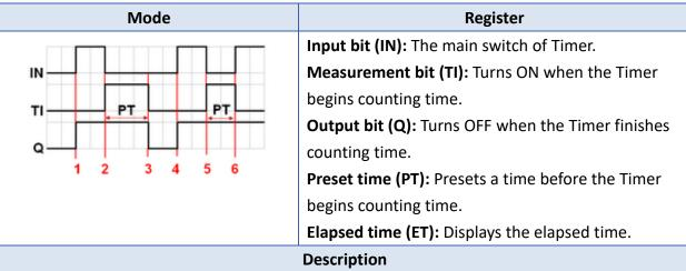
**Period 1**: When the IN turns ON, the TI remains OFF and the Q turns ON, the ET is reset to 0.
