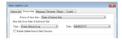
Option List object can be used with historical data display objects, such as Trend Display object, History Data Display object and Event Display object to control which history file should be shown. The figure below is an example of Option List used with Trend Display.
