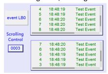
If [Scrolling control address] is enabled, the scroll bar cannot be used for scrolling, but still shows the relative position of the content. If the control address holds a value that is larger than the total number of lines, the display will stroll to the end. Please note that with this address enabled, the horizontal and vertical scroll bars will not be available on the object; please make sure that the width of the object is enough for completely showing the content.
