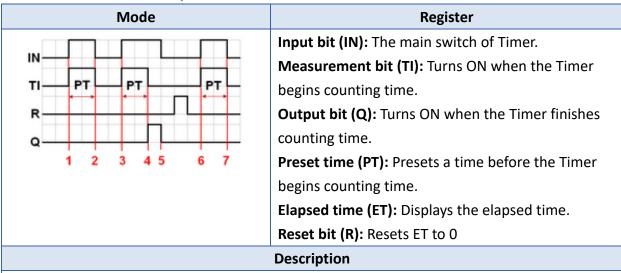
**Period 1**: When the IN turns ON, the TI turns ON and the elapsed time ET starts counting, the Q remains OFF.
