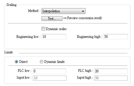
Click [Test] button to preview the result of Interpolation. Enter a value in [PLC] field as shown in the following figure, for example, enter value 15, and the result, which is 40, will be displayed.
