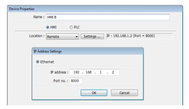
**3.** Create a Set Bit Object, select "HMI B" in [PLC name] to control the address of the remote HMI.
