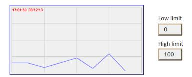
To zoom in the Trend Display, enter a value less than 30 in [High limit] as shown in the following figure.
