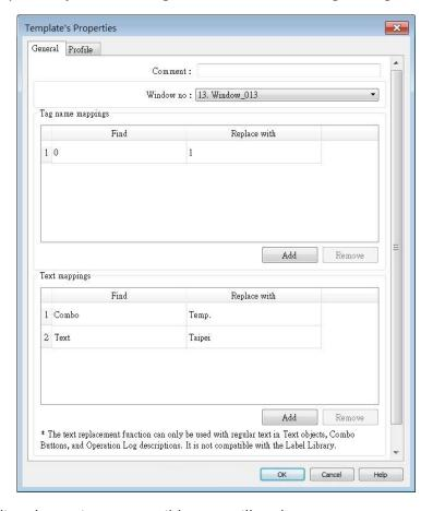
8. After compiling the project, EasyBuilder Pro will replace any tag names containing "0" with "1" for objects in the Template Window that use them. This means that "Tab\_0" will be replaced by "Tag\_1". The text mapping feature will also replace object comments, text contents, and text labels according to the settings defined in the Template object.
