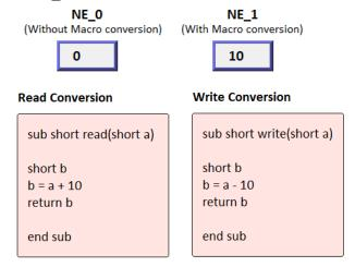
Enter 80 in NE\_1, [Write conversion] is executed and the value gained will be 70. NE\_0 displays 70.
