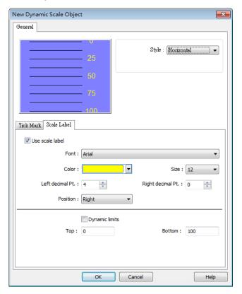
Set the font, font color, font size, and decimal point of the scale label. Set the position to display the scale label.
