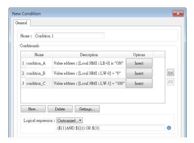
2. Now the Condition objects can do the same thing as the macro, which triggers actions according to the conditions.
