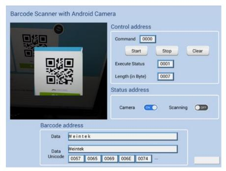
4. If the size of the data read exceeds the maximum allowable size set in Read Byte Limit (10 bytes in this project), the Execution Status turns to 2 (error code). The exceeding part will still be displayed in the ASCII objects in Barcode Address group box, since the data length displayed depends on the ASCII object settings (20 words in this project).
