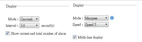
When [Carousel] mode is selected, the option to display the current and total alarm count and set the interval in seconds can be enabled.
