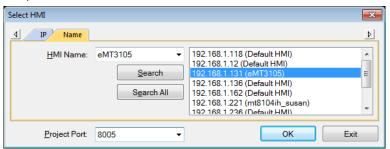
The three consecutive ports of the project port no. are preserved for HMI communication. In the setting above as an example, Port No. is set as 8005. Port 8005, 8006 and 8007 should be reserved. In this case when executing simulation on PC, please make sure that these ports are not occupied by other programs.
