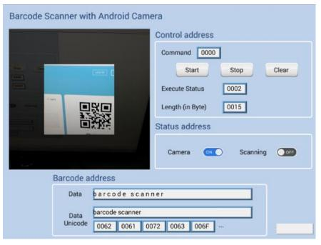
5. After changing to another page, Scanning turns OFF, the parameters are reserved. The parameters will be cleared when next time Start button is tapped, or Clear button is tapped.
