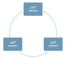
One cMT / cMT X HMI can be simultaneously controlled by multiple cMT Viewer clients. To ensure system safety by preventing an object to be controlled by multiple clients simultaneously, a control token can be set. Only one cMT Viewer client can acquire the control token at a time, and only the cMT Viewer client that acquires control token can operate the object. The rest of the clients can acquire the token one by one when the token is not occupied.
