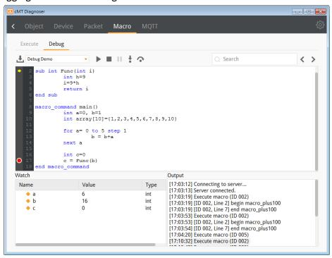
7. Click the Step Over button to run the macro line by line. Now, if the line contains a function, the result will be returned without debugging each line within the function call. When debugging meets a Breakpoint within the function call though, it stops there.
