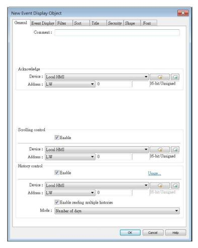
For cMT / cMT X models, only events with "save to history" option selected in the Event (Alarm) Log settings can be displayed in the Event Display object. The events that are not set to be saved in the history can be displayed using the Alarm Bar or Alarm Display object.
