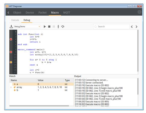
6. Click the Step Into button to run macro debugging line by line. If the line contains a function, cMT Diagnoser will enter the called function and continue line-by-line debugging from there. Changes of values can be observed in the Watch table.
