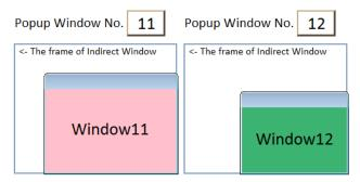
To close the pop-up window, apart from entering 0 in the designated word register, another way is to place a Function Key object in the pop-up window, and set the key to [Close window].
