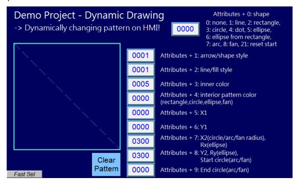
5. Press Clear Pattern button, and enter 3 in LW-0, a circle is drawn, and entering different values in LW-1~9 can change the style, the color, and the position of the circle.
