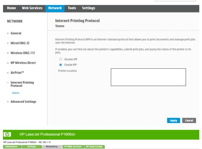
After enabling these options, available printers for installation can be found through the "Install network printer" list in HMI system settings, where "(IPP)" indicates the use of this protocol for communication.
