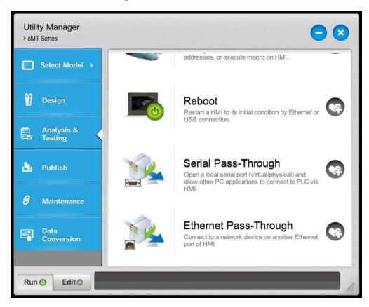
2. Click [Ethernet Pass-through] and then fill in the communication parameters.
