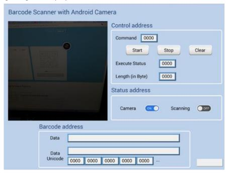
**2.** Tap Start button, the status of Scanning turns ON, the display turns bright, and is ready for scanning.
