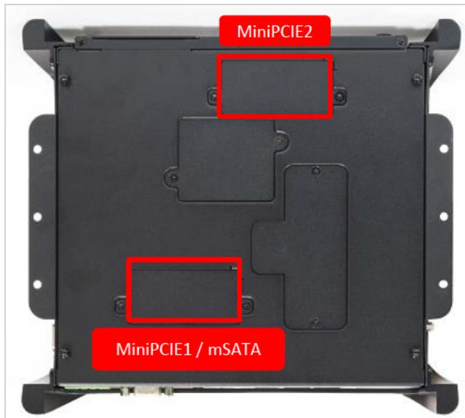
2. Insert mini PCIe card or mSATA module from 45 degree direction.
