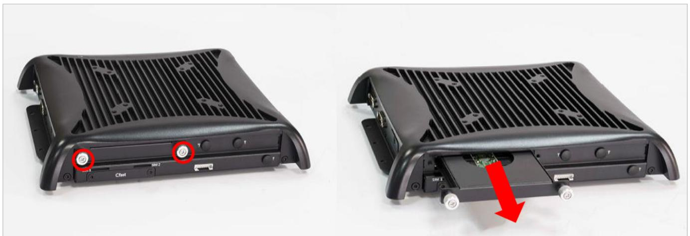
3. Lock the 2.5" HDD with HDD bracket using four screws (M3x4L).
