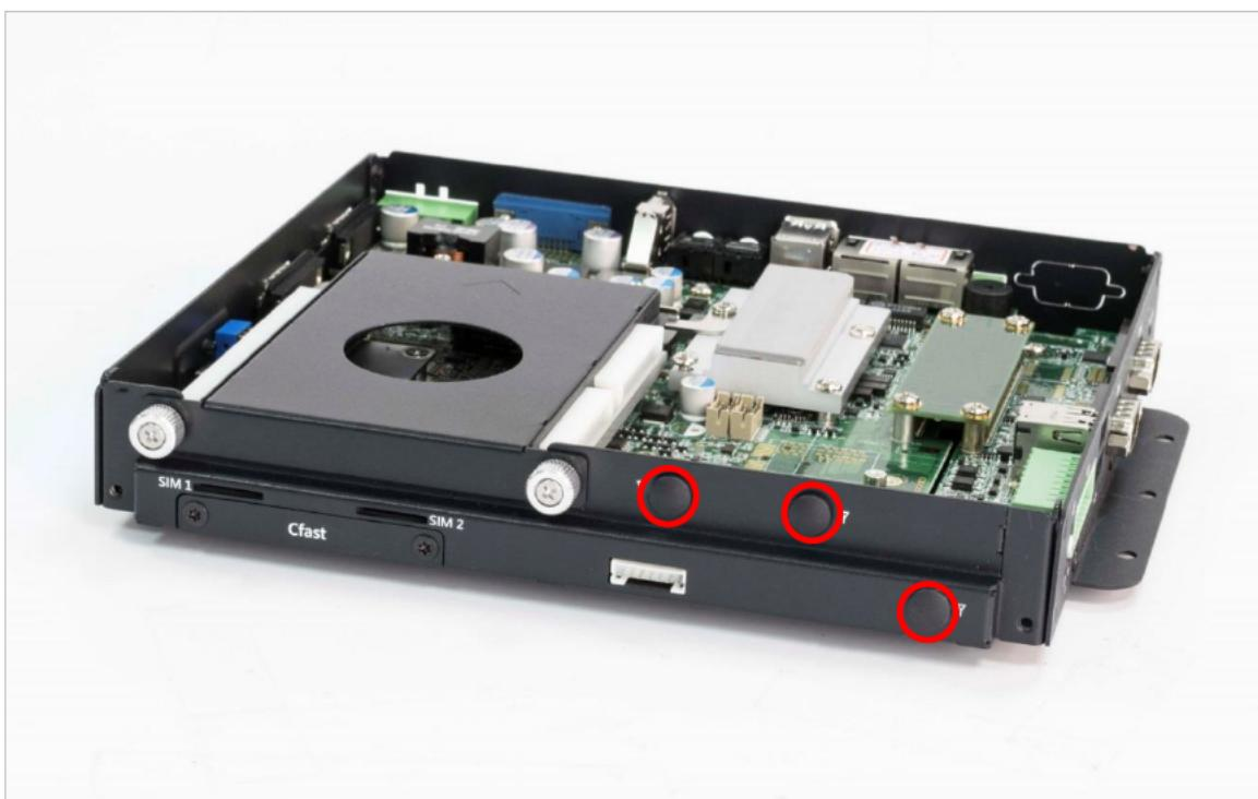
2. Remove antenna hole cover on the system panel.
