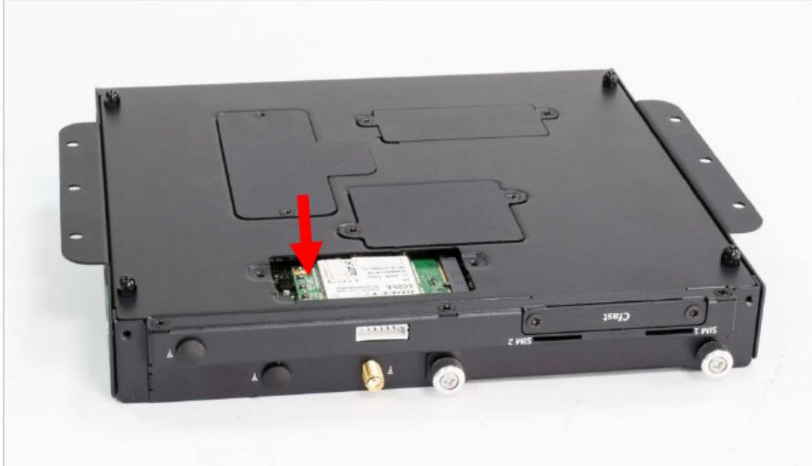
6. Assemble the antenna and antenna jack together.
