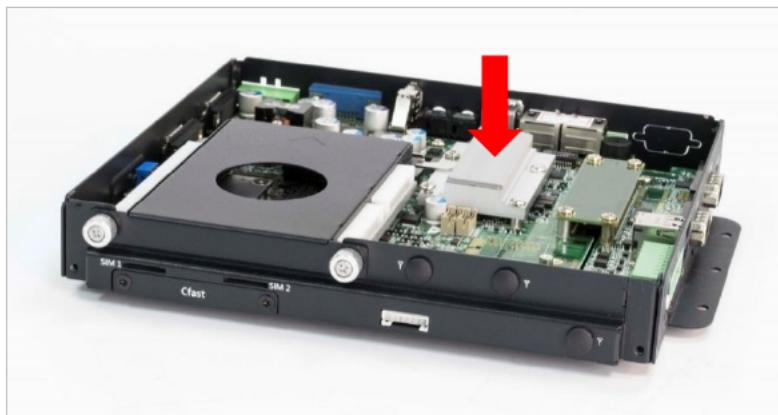
2. Close the chassis top cover following the below direction and make sure the aluminum part on the top cover is touching the thermal pad on CPU thermal block.
