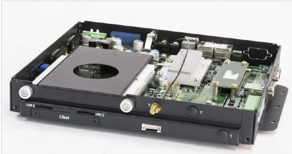
5. Attach the RF connector at the cable-end onto the communication module.
