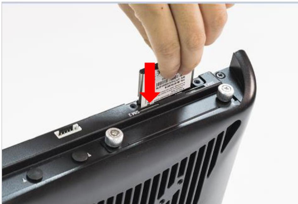
3. The socket is push-push type. Push the installed CFast card again to remove it.
