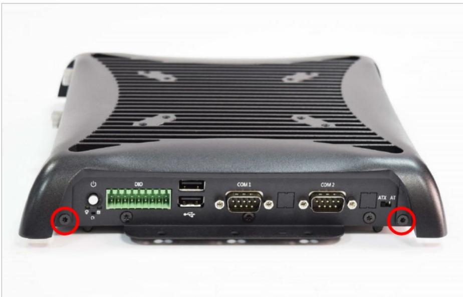
2. Remove the top cover of PC module.
