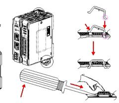
Rail mounting: DIN rail 35mm.
