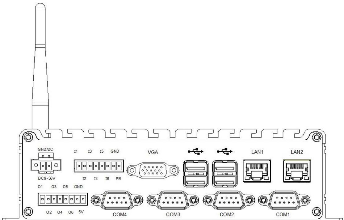
Figure 2.1.3.a2 Back panel of IFC-BOX2800
