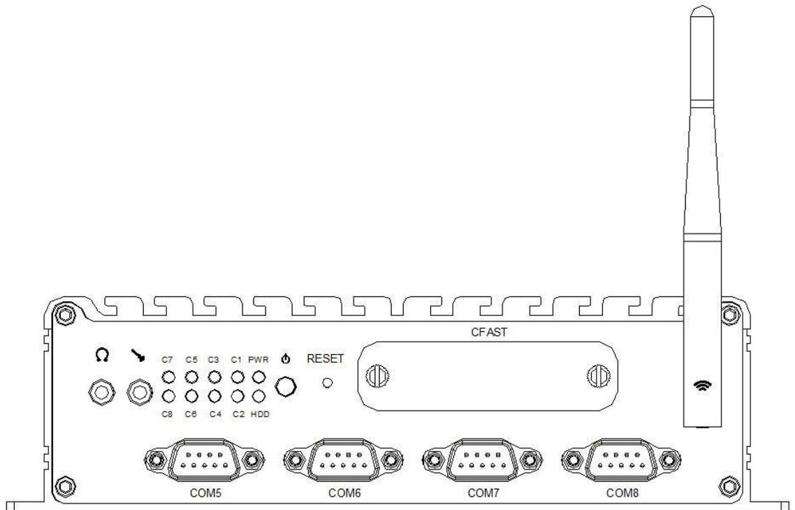
Figure 2.1.3.a1 Front panel of IFC-BOX2800
