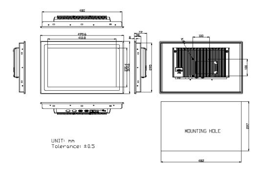
Figure 1.8: Dimensions of ARCHMI-818(P)H
