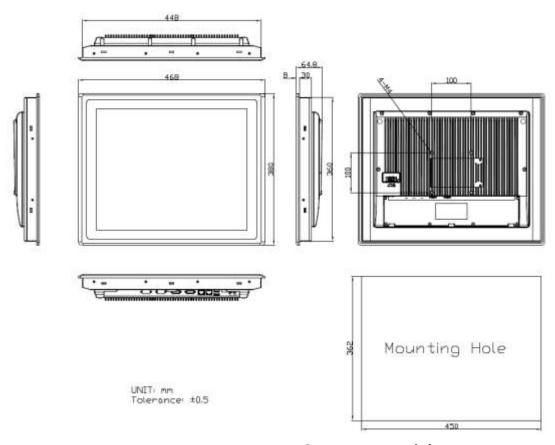
Figure 1.9: Dimensions of ARCHMI-819(P)H
