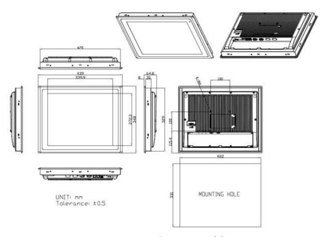
Figure 1.7: Dimensions of ARCHMI-817(P)H
