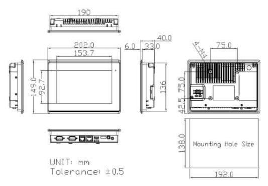
Figure 1.1: Dimensions of ARCHMI-807(P)H
