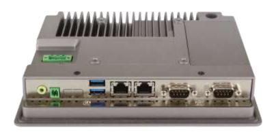
Figure 1.12: Rear View of ARCHMI-807(P)H
