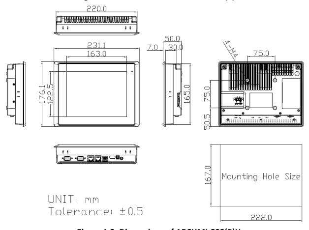
Figure 1.2: Dimensions of ARCHMI-808(P)H
