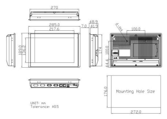
Figure 1.3: Dimensions of ARCHMI-810(P)H
