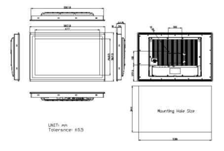
Figure 1.10: Dimensions of ARCHMI-821(P)H
