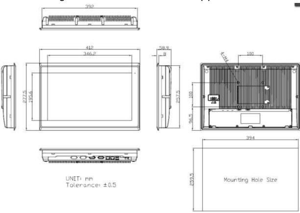
Figure 1.6: Dimensions of ARCHMI-816(P)H
