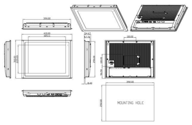
Figure 1.5: Dimensions of ARCHMI-815(P)H
