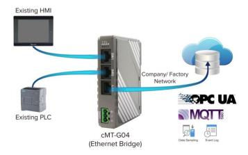
cMT-G04 can be configured by the following ways. Way1. Connect cMT-G04's LAN port with a PC, and on the PC open a web browser and then enter: <a href="http://169.254.0.1">http://169.254.0.1</a>, password: 111111.
