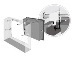
Minimum required clearances (along the overlay): Top / Bottom / Sides 15 mm Maximum panel thickness: 4.5 mm
