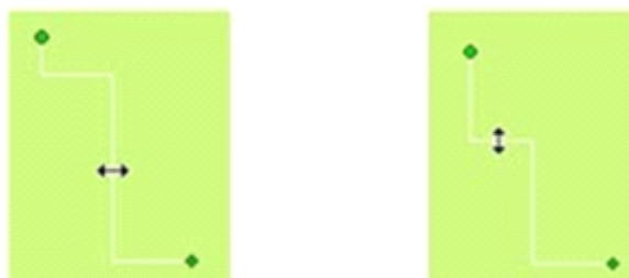
Figure 4-33: Modifying a straight connection line
