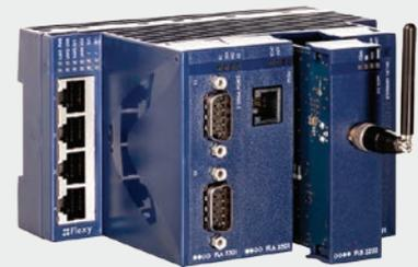
The eWON Flexy is the first industrial modular M2M router and data gateway designed for OEMs and system integrators. The flexibility allows remote devices to be linked in an environment where communication technologies are constantly changing, and lets you communicate universally with the most varied field equipment, regardless of the protocol used.
