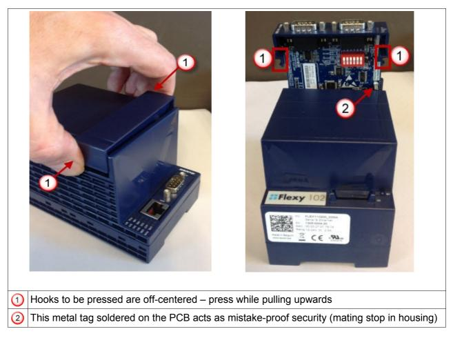
Insert the Extension Card carefully and slide it down until the hooks are *clicking*. Make sure the card is completely inserted. **DO NOT insist** if you feel some resistance when trying to insert the card. It probably means you are trying to insert the card in a wrong slot. In such case, check slot compatibility of the relevant Extension Card.
